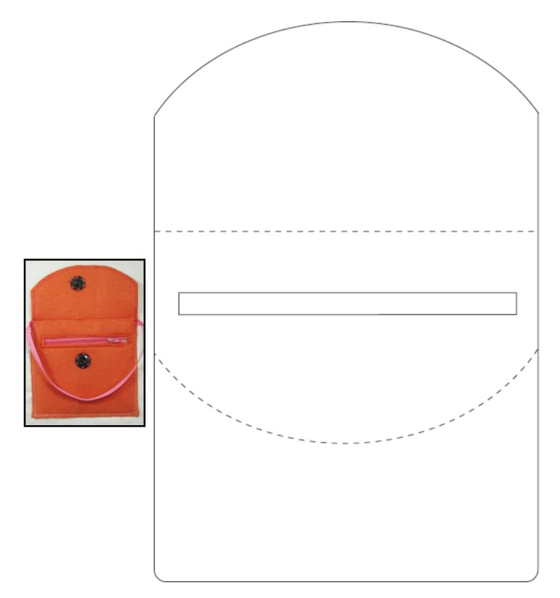
The purse is made with a double layer of felt. Cut the center rectangle out and add a zipper. Zig zag the moveable flap. Zig zag the lower part of the purse to the page. Straight stitch across the base of the flap. Add a snap for a closure.
