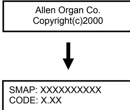
**Note:** The LCD will display the current stopmap level (SMAP) and operating software base code level (CODE) currently installed in the organ.
